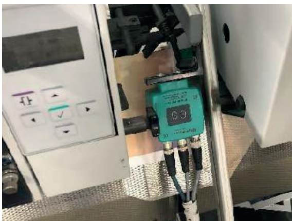
→ Camera including mount on a folded sheet feeder of the Stitchmaster ST 450 saddle-stitch machine
