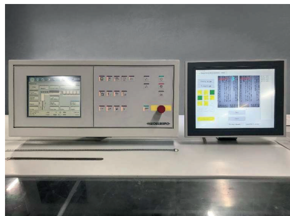
→ Panel PC next to the control panel of the Stitchmaster ST 450 saddle-stitch binder
